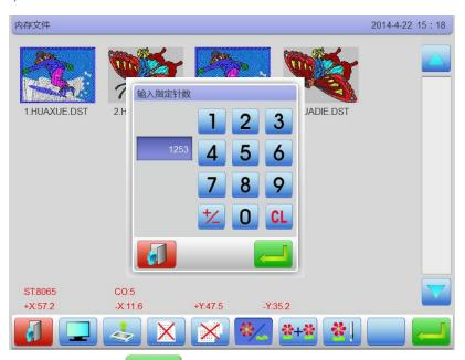
Input the needed stitches, click , the interface will switch to confirm segmentation, After finishing, it'll automatically return "Cut Designs" interface.
