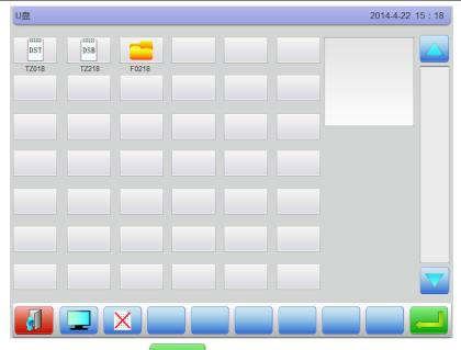
Click the requested design, press, automatically show the download progress and memory No., after finishing, will automatically return U disk operation interface, continue to do the next.
