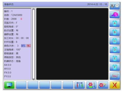
Choose the current selected frame type, when choose cap frame and A-E frame, it'll automatically find the absolute origin, and stop the center of the frame, please note frame move. The center and the range of cap frame and A-E frame refer to the frame setting. "Other" frame don't find absolute origin, the embroidery range will be defined by software limit (the details refer to software limit setting).
