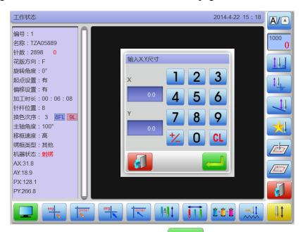
Writing the needed size of XY direction, click it'll pop-up a dialogue generated finished, switch start embroidery, when completed, the frame will automatically return the current design's origin to stop, and then can do the other operation.
